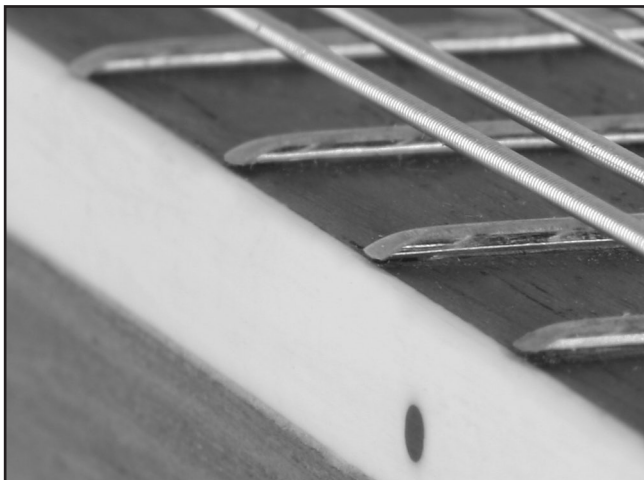
Figure 19. Example of correctly angled fret ends.
